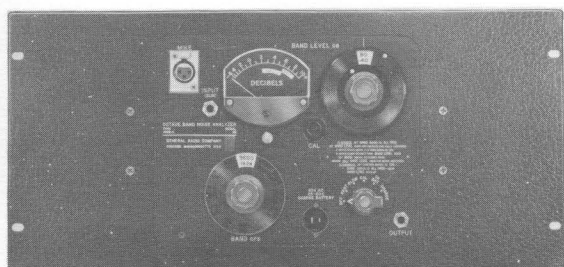
Figure 1-1. Views of the Type 1558-A Octave Band Noise Analyzer. (Above, left) in relay-rack adaptor; (above, right) case closed; (right) with microphone attached; (below) panel view.
